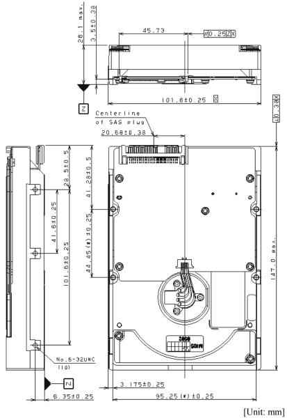
(\*) is a dimention between the screw holes for the bottom mouting.
